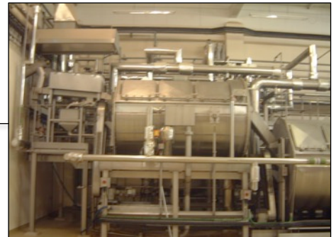
Pre cook rehydrates product and pre heats the wheat, reducing load on main cooker
