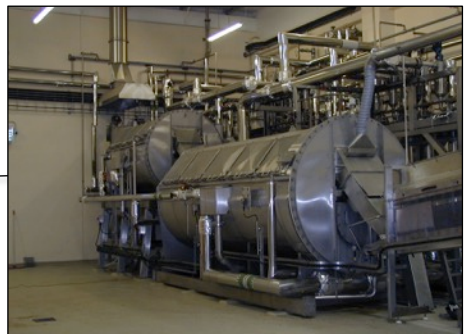
Main cooker, temperature and time controlled process, minimal hydration occurs here
