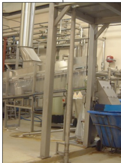
Discharge Conveyor distributes product for further processing
