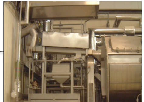
De-stoner removing foreign objects from the product before cooking commences
