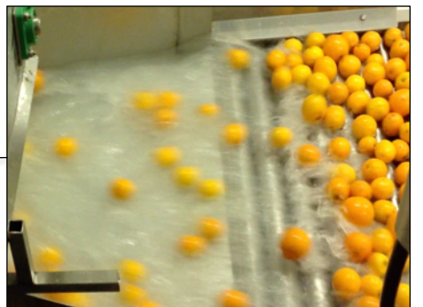
Discharge from pipe washer on to roller spreader conveyor.
