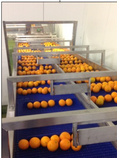
Elevator transfers product to high level juicer units
