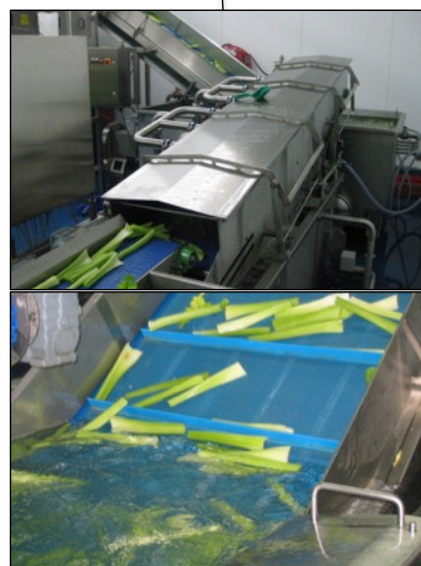
2 stage wash process. Spray wash to remove tough grit & dirt. Flume washed for fine clean & sterilization
