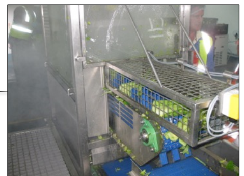
Water jet cutting, cuts through the head and heart to produce celery sticks
