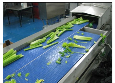
Inspection conveyor means all waste can be removed before further processing
