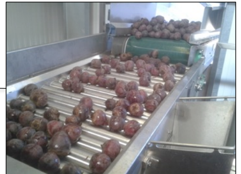
Bulk feeds roller inspection conveyor, product checked and removed if defective
