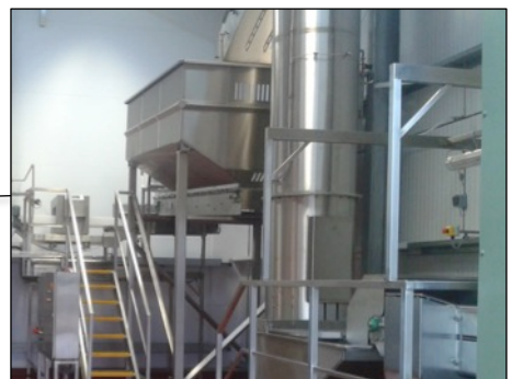
Stones are removed from product flow in a vertical de-stoner
