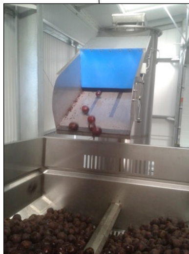
The vertical de-stoner elevates the product up to another bulk hopper
