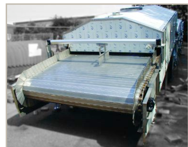
COATING DRYER FEED END (under construction)
