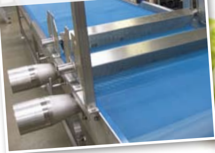
CONVEYOR WITH AIR KNIVES AND SUCTION PLENUMS - air knives and plenums are all adjustable to provide a perfect balance
