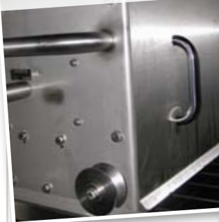
OIL WEIR SYSTEM INSTALLED - travel locking and guide raising and lowering handles easily accessible on the side of the unit
