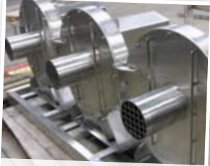
AMBIT STAINLESS STEEL FANS - Fans serving the air knives and suction plenums
