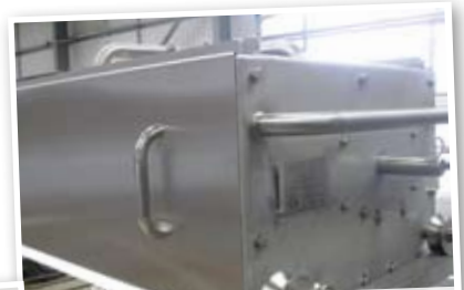
END VIEW WITH COVERS - dismantlable covers for cleaning once unit is removed from over the fryer
